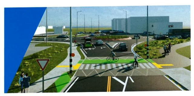
11.14.4 Pedestrians (Slip lanes): Crossing slip lanes can be very difficult for pedestrians, especially vulnerable road users, as drivers are preoccupied with looking at traffic flows. Consideration needs to be given to installing raised platforms and pedestrian crossings so that pedestrians can cross roads as safely
